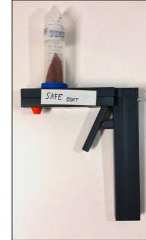
Fig 2: The newly designed 'food gun', or aquatic food dispenser. The falcon tube on top can be removed and refilled with dry food as needed. The trigger will release food that is equal to 5% body of 15 fish
